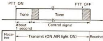
When the OFFSET switch is ON, the control signal is transmitted about 1 second after the PTT switch is activated. This delay prevents the control signal from being broken by the slow response of some repeaters.
