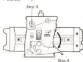
4. Press the lever down to secure the transceiver.
