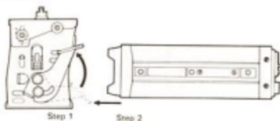
3. The angle of the bracket may be adjusted to any of 5 possible viewing angles by loosening the 4 allen bolts at the top of the bracket using the hex wrench provided.
