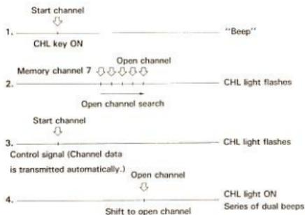
1. The frequency displayed when the CHL key is pressed is stored in memory as the start channel.
