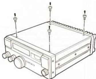
attaching the cover, be sure not to let the wiring be caught between the covers and chassis. Be sure to plug in the speaker connector on the bottom cover.
