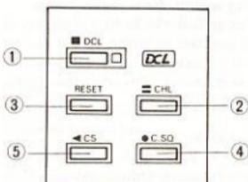
① DCL (Digital Channel Linkage) key
